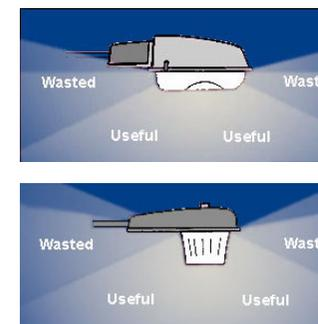
These **semi-cutoff** lights are fitted with drop-lenses or refractors that emit a greater portion of their light sideways for wider road coverage but create more glare. They also send light upwards that contributes to skyglow. Full cut-off fixtures should be considered as an alternative. Mercury lights (bottom) are a bad choice. They are especially glary and inefficient compared to other lights and their used should be discouraged.
