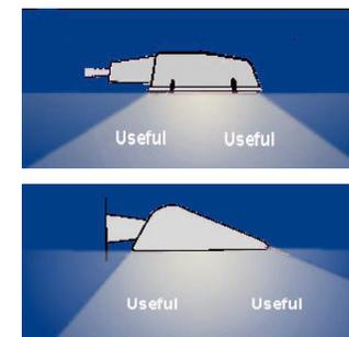
**Full cut-off** fixtures direct light below the horizontal. At top is one of the standard "cobra head" fixtures fitted with a flat glass. It aims light downward and sideways avoiding uplight and glare that improves the quality of lighting. The floodlight (bottom) is mounted in the horizontal position for security lighting and areas such as car yards and parking lots.
